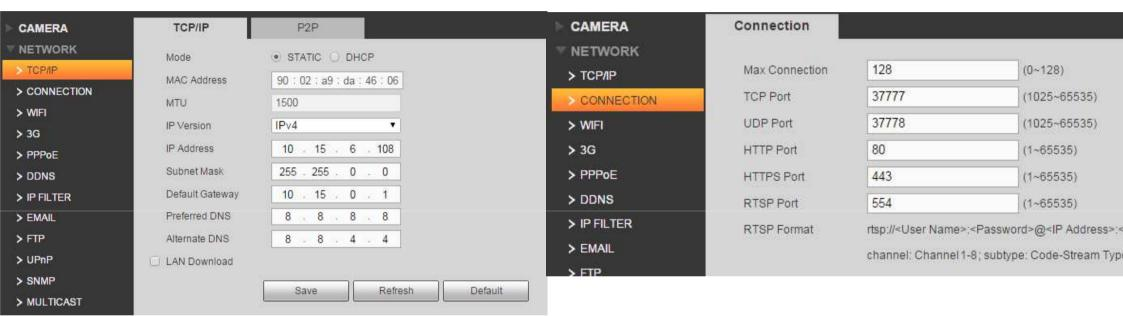
Check the IP address and the port number of the DVR/NVR.
