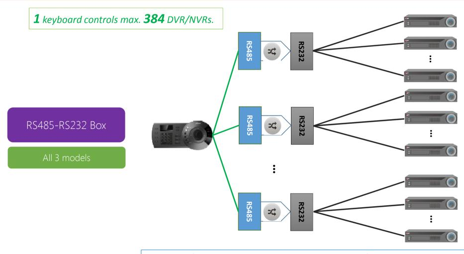
1 keyboard  $\rightarrow$  32 RS485-RS232 boxes, 1 RS485-RS232 box  $\rightarrow$  12 RS232 connections
